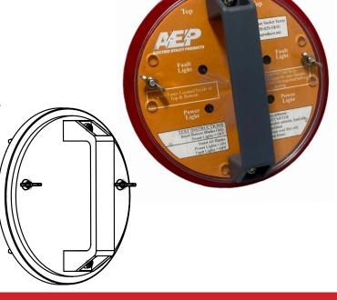
The AE Products Single Phase Socket Tester detects short circuits, backfeed and wiring errors in a 120/240 Volt, 3-wire, single phase, self-contained socket. This unit is equipped with high intensity power and fault lights to indicate whether or not the meter is safe to install. The heavy duty handle allows for quick and easy installation.
